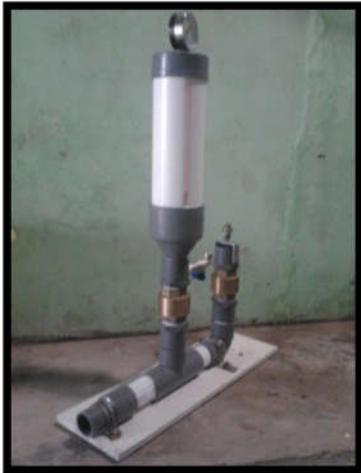
Gambar 3.2. Pompa Hidram
