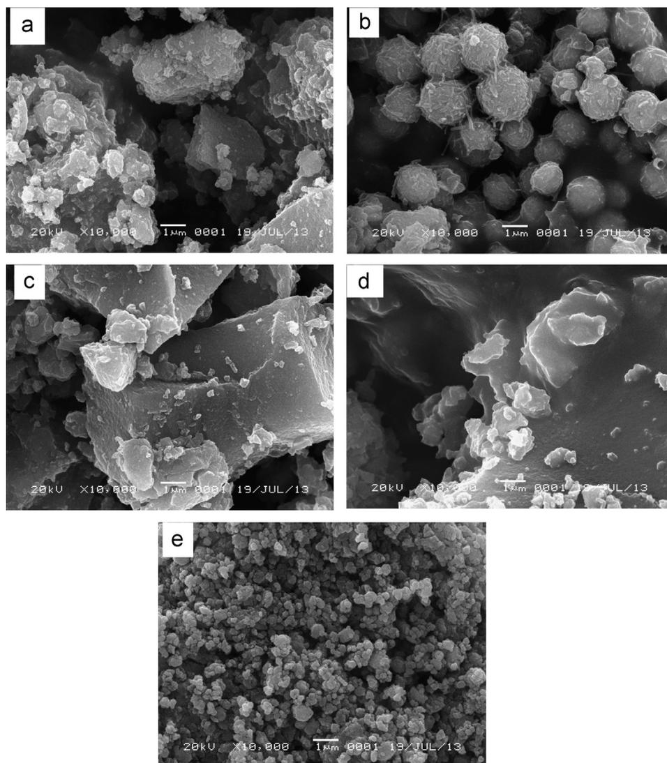
**Fig. 2.** Scanning electron microscope images of ZnO nanoparticles with various concentrations of *S. rarak* rinds extract of 0%, 2.5%, 5%, 7.5%, and 10%.
