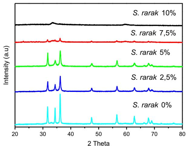
**Fig. 1.** X-ray diffraction pattern of ZnO with various concentrations of *S. rarak* extract of 0%; 2.5%; 5%; 7.5%; and 10%.
