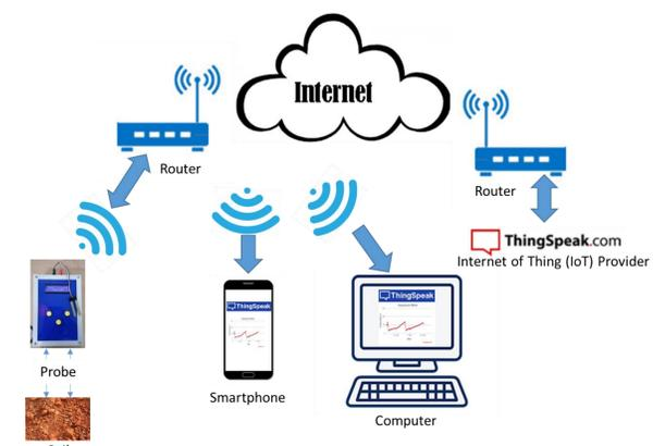
Figure 4. Future development of the remote instrument for temporal soil water measurements.
