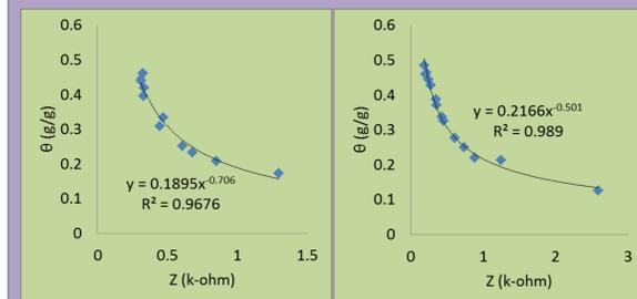
Figure 3. Typical non-linear models to predict temporal water content ( $\theta$ ) from electrical impedance ( $Z$ ) at repacked soils.
