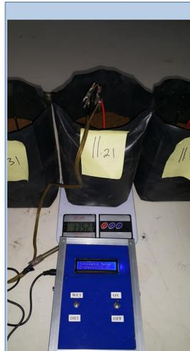
Figure 2. Instrument used to measure  $Z$  and balance to measure water content
