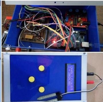
Figure 1. A portable impedance meter using auto-balancing bridge.
