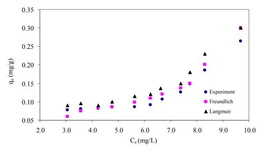
Fig. 9: Fitting of Langmuir and Freundlich isotherm into the experiment data for SD
