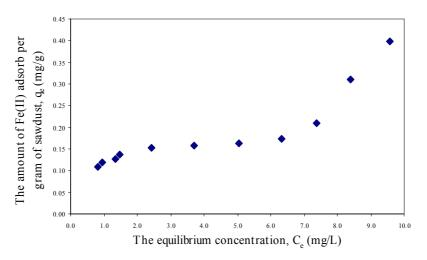
Fig. 4:  $q_e$  vs.  $C_e$  (batch test) by using SDC
