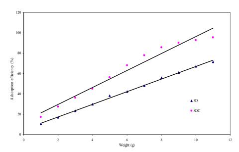
*Fig. 2:* Adsorption efficiency of Fe (II) using SD and SDC 224
