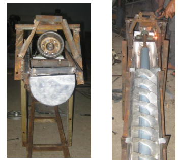
Figure 5. Assembly of Magnet Motor on Screw Turbine
