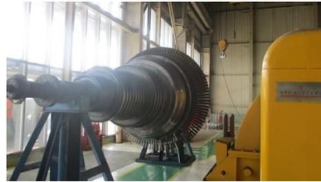
Gambar 2.7 Rotor Turbin
