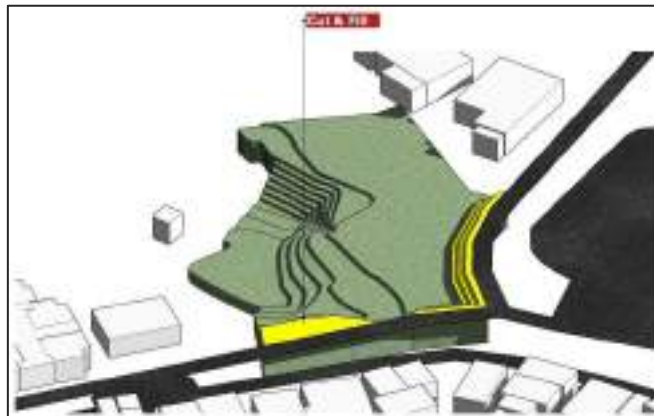
Gambar V. 37 Cut and fill
