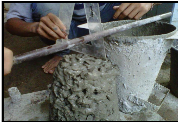
Gambar 4.10 Proses Pengujian Slump
